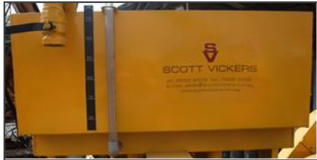
Water Tank with Level Gauge
