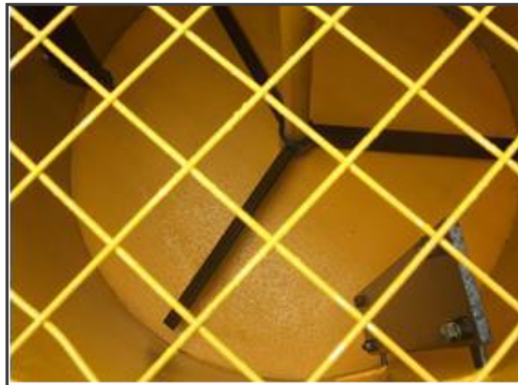
SV60 Impeller & Baffle Plates
