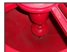
Bearing-free mixing system
