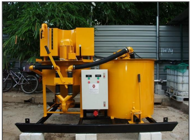
SV6065E Electrically-operated SV65 High Speed Colloidal Grout Mixer complete with Dust Extraction Hood, SV60 Low Speed Grout Paddle Mixer, all mounted on a Skid Chassis with Lifting Eyes. Control Panel with Inverter to provide SV65 with two-stage speed for use with OPC and Micro-fine cement.
